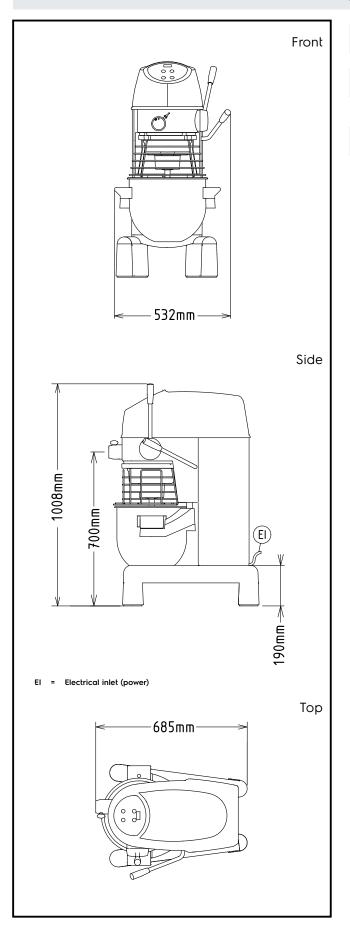
Electric Supply voltage: 208-230 V/1N ph/60 Hz Capacity: Performance (up to): Capacity: 20 litres **Key Information:**
